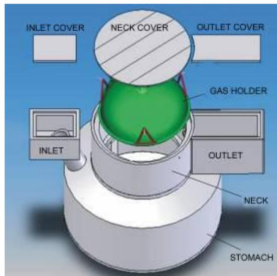
The pressure is caused by the distance between water level of gasholder and water level of concrete tank. The advantages of Puxin biogas digester:
